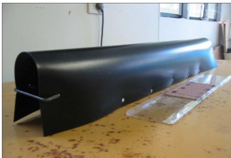
Tracking tunnel showing strong plastic cover with extra length and a metal bracket to prevent possums, weka and kea tampering with monitoring card. DOC
